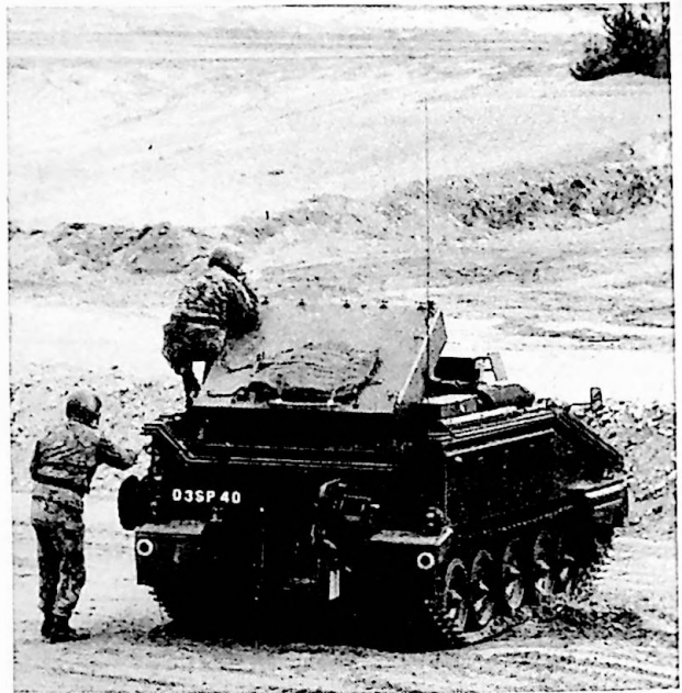
Swingfire long range anti-tank missile launcher on a Striker armoured tracked vehicle
