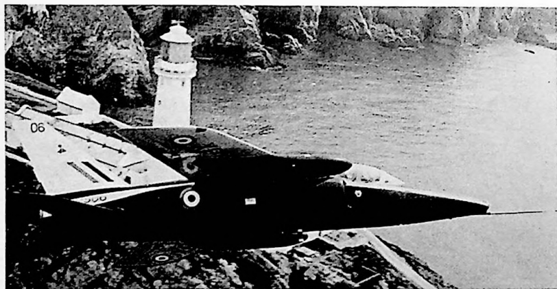
Fig. 5 The Hawker Siddeley Gnat, used as a trainer and by the Red Devils acrobatic team
